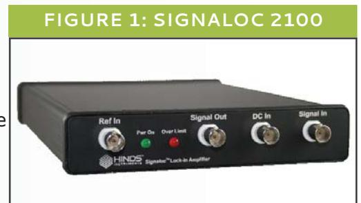
The display is virtual, as shown in Figure 2. Information is sent from the lock-in amplifier to a computer via RS-232 where it is displayed and available for immediate, real-time analysis by the user's program.
