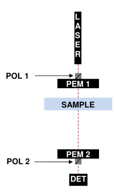
Figure 1.2 Optical components of system
