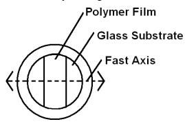
Figure 5.1 Fast Axis Orientation of Polymer Film Sample
