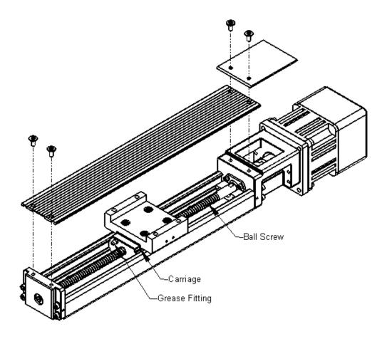
Figure 5.3 X-Rail & Y-Rail Lubrication
