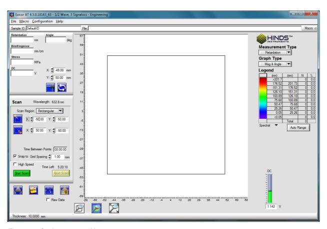
Figure 3.4 Setting up a 100 X 100 mm scan
