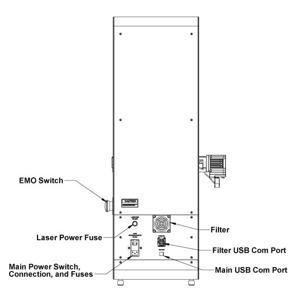
Figure S.3 Rear Panel Connections
