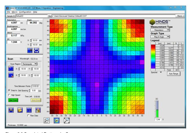
Figure 3.6 Completed Rectangular Scan
