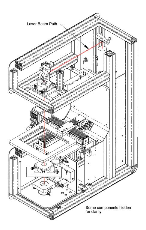
Figure S.1 Laser Beam Path
