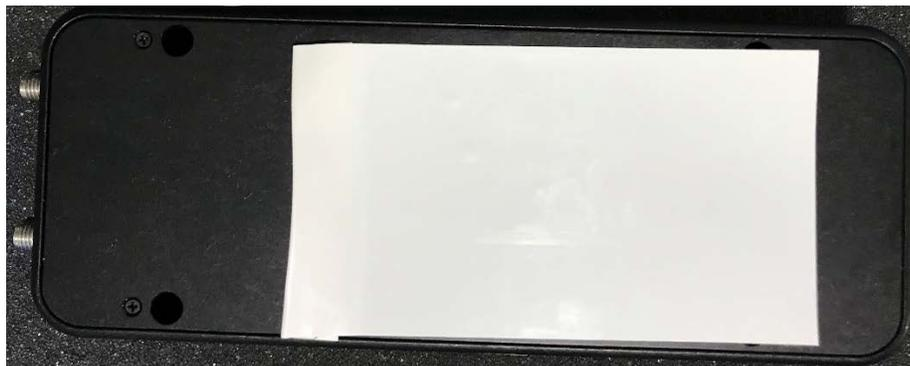
*Figure S.3 Removal of White Cover on Optical Enclosure*
