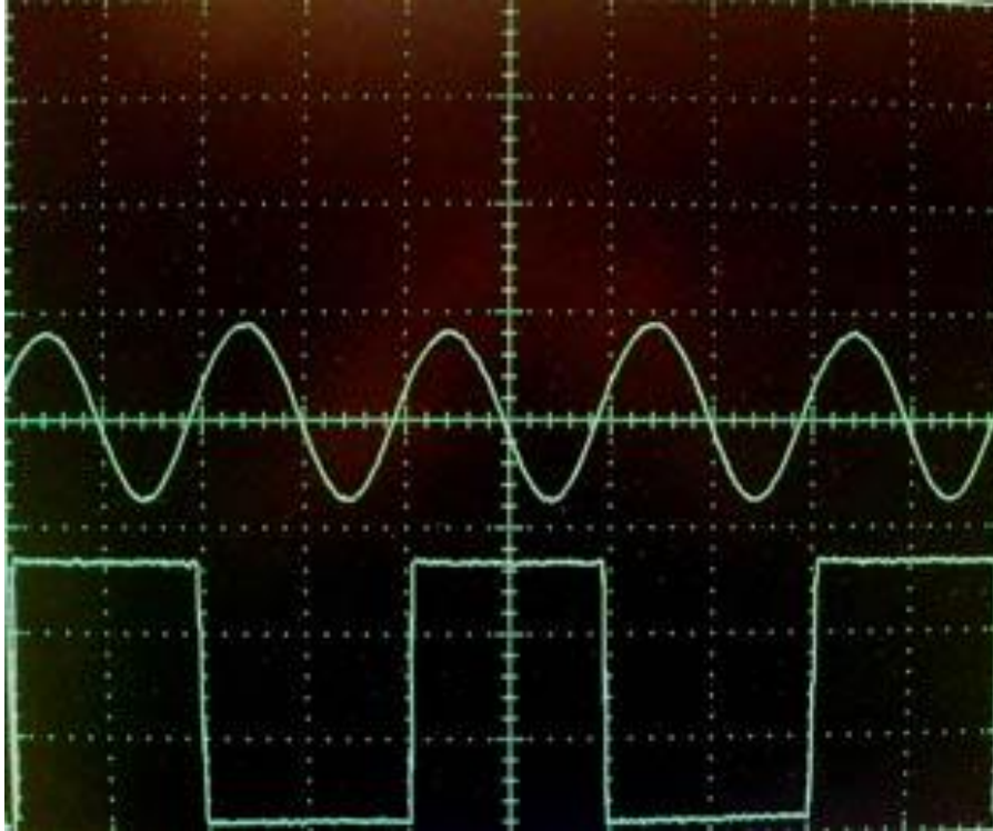
Oscilloscope Waveform for PEM Set to 0.25 Wave Retardation Between Crossed Polarizers and PEM 1f Reference Signal
