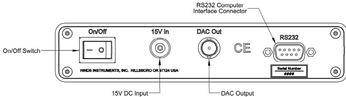
Figure 2.2 Lock-In Amplifier Module Back Plate
