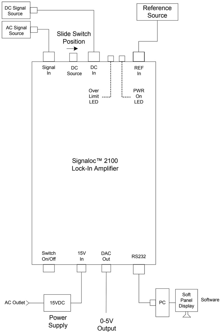
Figure 3.3 Measuring Split AC and DC Inputs
