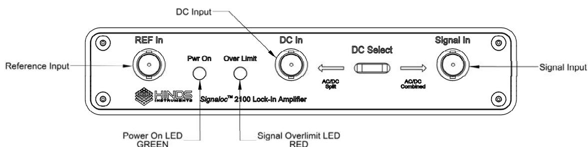
Figure 2.1 Lock-In Amplifier Module Front Plate
