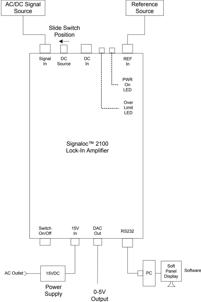
Figure 3.2 Measuring Combined AC and DC Input
