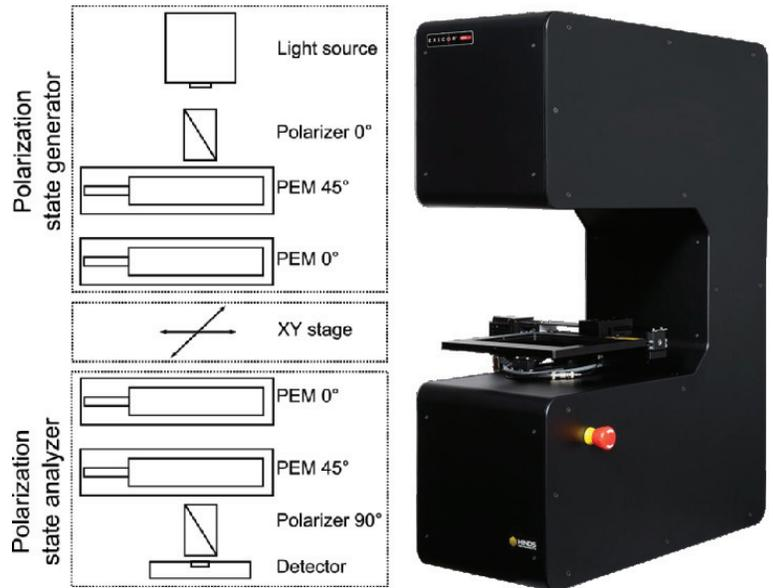
Figure 5: Hinds Exicor 150XT transmission Mueller polarimeter.
