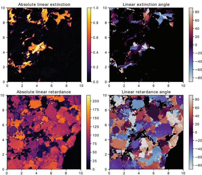
Figure 2: Linear extinction and linear retardance measured of petrographic thin section at 633nm using a Hinds Exicor 150XT transmission Mueller polarimeter.
