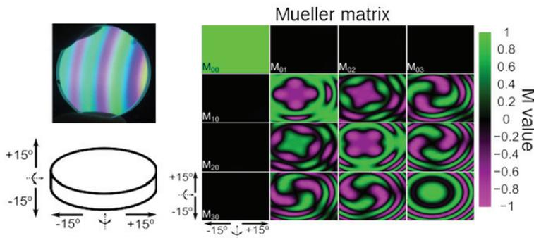
Figure 3: Mueller matrix of c-cut quartz at 633nm using a Hinds Exicor 150XT transmission Mueller polarimeter.
