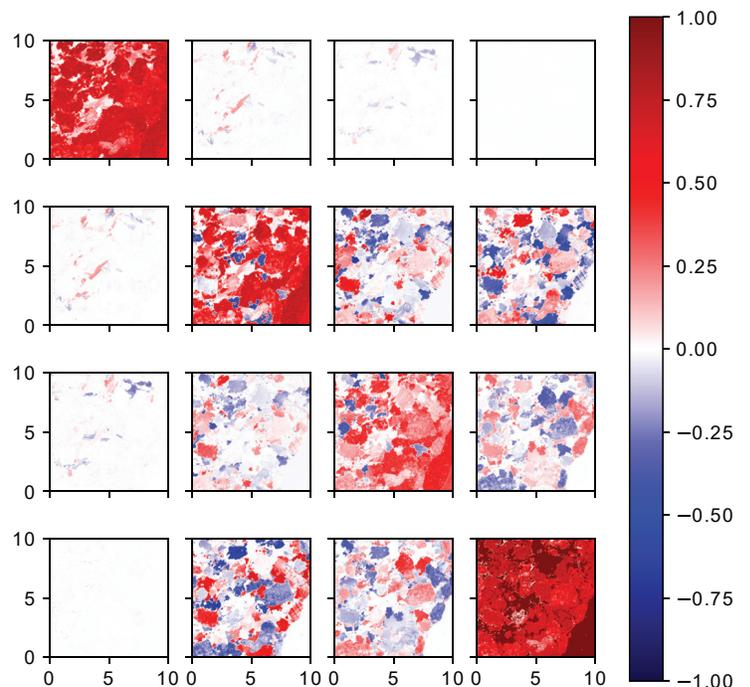
Figure 1: Mueller matrix of petrographic thin section at 633nm using a Hinds Exicor 150XT transmission Mueller polarimeter.
