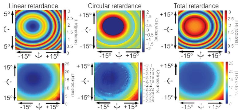
Figure 4: Absolute linear retardance, circular retardance, and total retardance of c-cut quartz at 633nm using a Hinds Exicor 150XT transmission Mueller polarimeter.
